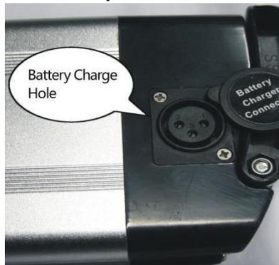
2. Insert the charging plug of recharger into the battery charge hole; pay attention to the plug direction, please do not insert or dismantle by force.
