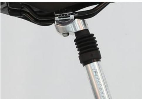
4. Push the side position of the saddle head and the upper part by force; if the saddle is not stable, please first check whether the saddle clamp is locked. If so, please repeat the operations above.
