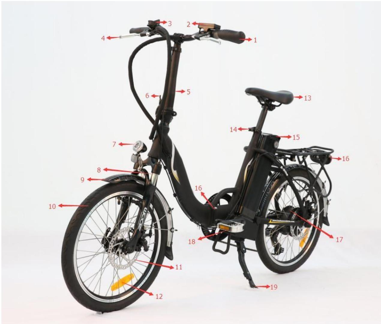
1. leather handle 2. LCD display 3. Shimano Shifter 4. Brake lever 5. stem 6. Stem folding clamp 7. LED light 8. PET mudguard 9. suspension front fork 10. Wheel 11. Disc brake 12. Wheel Reflector 13. Saddle 14. Seat post clamp 15. Battery 16. Frame folding clamp 17. Motor 18. Pedal 19. Kickstand
