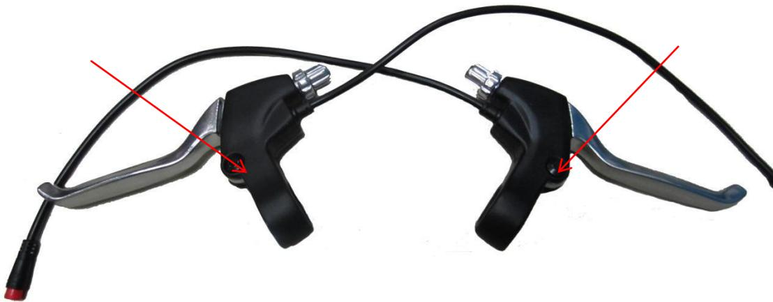
The effective stroke of the brake cable is about a half of the distance between the brake lever and the grip;
