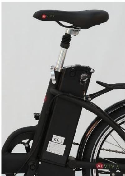
cylinder of battery pack are on, make the opening groove behind the battery pack align with the battery case slider, put the battery pack down into along the battery case slider until the discharge hole at the bottom of battery pack and the discharge plug of battery pack in complete contact, finally press slightly with key into the inside key, at the same time turn the key in a clockwise direction until the key cylinder go through the hole on the battery case slider, then loosen the key.
