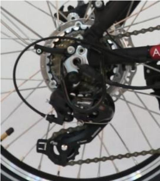
H bolt: when the chain speed changes to the biggest fluted disc, the chain will fall off, and the H bolt will be locked. But if it is too tight, the chain can't climb to the biggest fluted disc.
