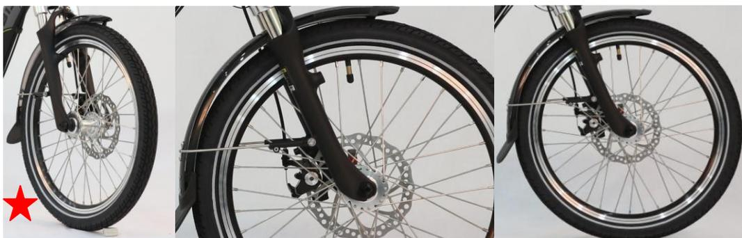
When fastening the nut for front wheel hub, press down the front fork appropriately so that the front wheel hub can work closely with the front fork.
