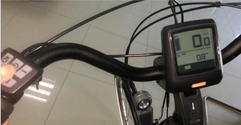
2. you can choose the mode according to the button, everything will show on the display. For speed, range, temperature, time and battery.
