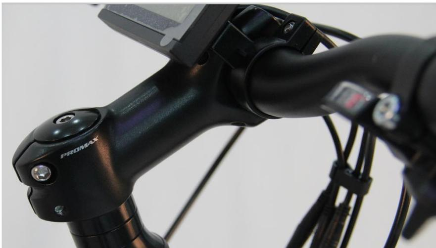
2. Unscrew the stem upper part, and put the handle bar inside, and then screw them tightly after adjust the handle bar at the right position.
